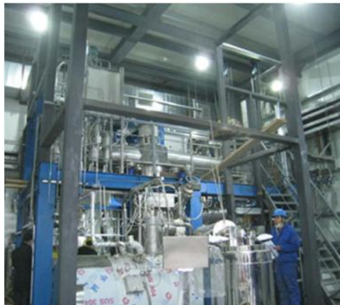
High-temperature fluoride salt experimental loop
