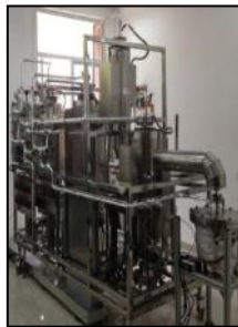
Prototype for molten salt production (10ton/y)
