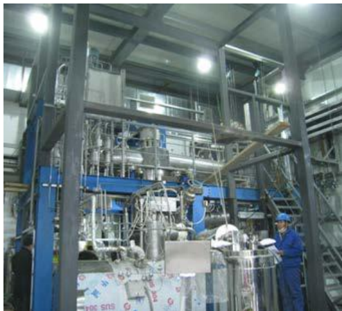
High-temperature fluoride salt experimental loop
